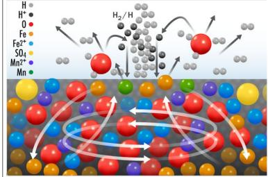
A schematic of the molecular interactions that take place during hydrogen-plasma-smelting-reduction of iron ore.
