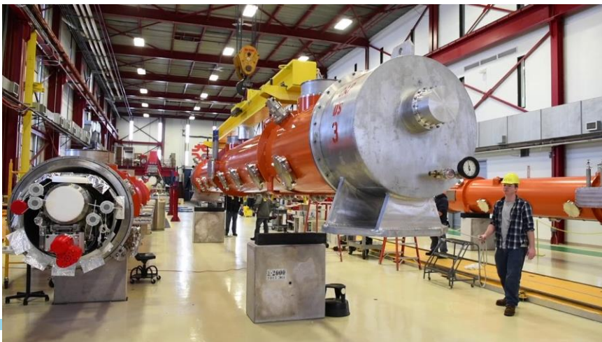
Cryomodule built at Fermilab for the new LCLS-II free electron laser light source at SLAC
