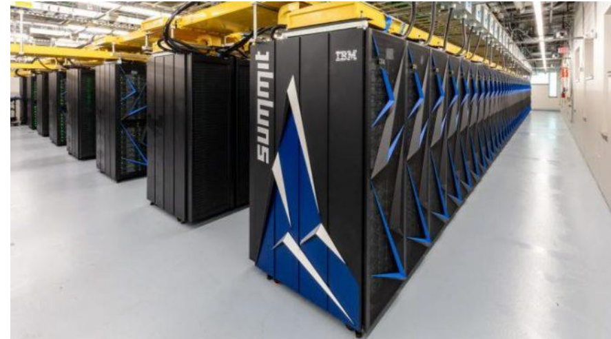
SUMMIT IBM, 4,600 Nodes 2 Power9 + 6 NVidia Volta Mellanox Network – Non-blocking Fat Tree ~200 PFLOPS, 13 MW
