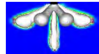
RANS calculation for fuel injector captures bulk behavior
