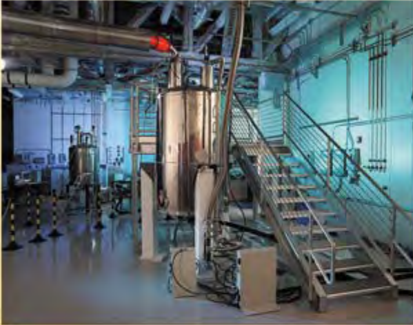
Environmental Molecular Sciences Laboratory's 800-MHz nuclear magnetic resonance spectrometer at Pacific Northwest National Laboratory
