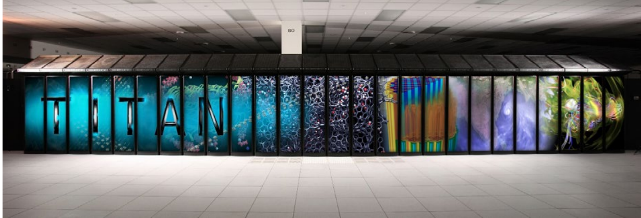
By upgrading its Jaguar machine and installing NVIDIA GPUs, ORNL created Titan, which reclaimed the No. 1 position on the TOP500 List.
