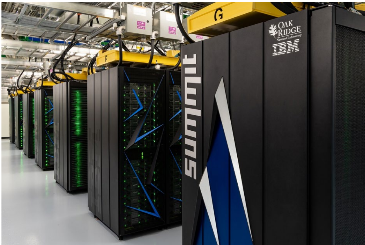
Installed in 2018, Summit at the OLCF has held the No. 1 position on the TOP500 List four consecutive times. Using IBM Power9 CPUs and NVIDIA Tesla V100 GPUs, Summit achieved performance of 148.6 petaflop/s.
