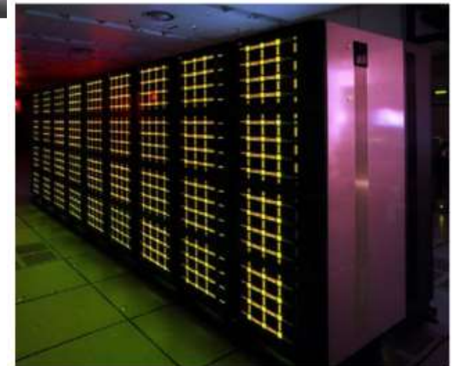
to address the grand challenge applications listed ORNL's Intel Paragon system was installed in 1995, comprising 3,072 processors to support research into Grand Challenge problems.
