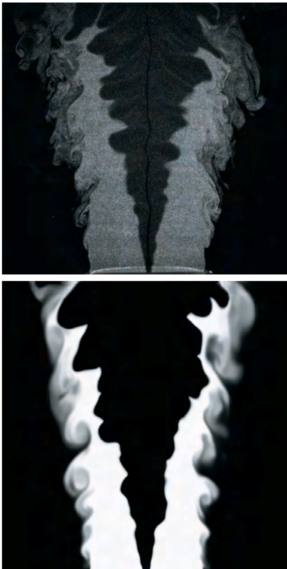
Figure 7. Comparison of experimental particle image velocimetry crossview of the turbulent “V” flame (top) and a simulation (bottom).
