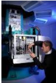
Core facility - Geocentrifuge (2m radius, 50 g-ton capacity) enables unsaturated flow experiments
