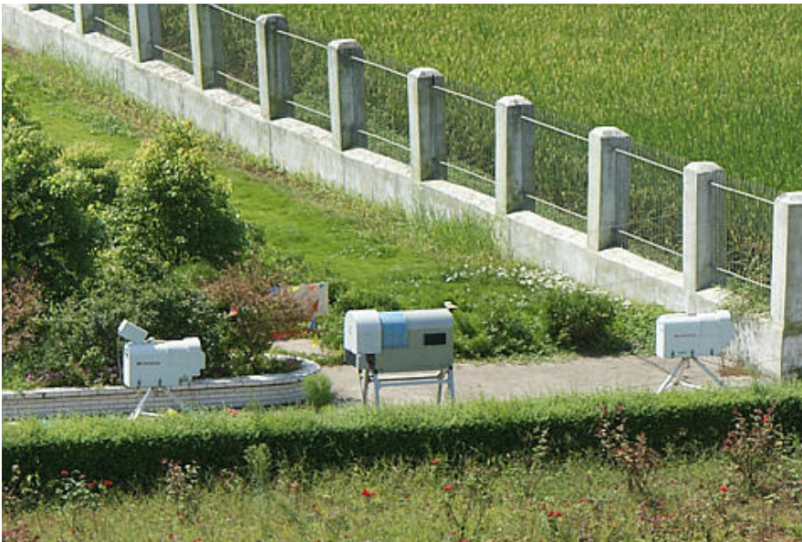
Shouxian instrument deployment, from left to right: microwave radiometer profiler, high-frequency microwave radiometer, and microwave radiometer.
