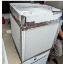
Affordable Indoor Air Filter (Corsi-Rosenthal Box)
