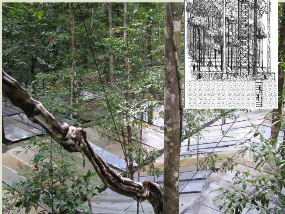
Fig. 5.2. Drought Experiment Infrastructure at Tapajós and Caxiuanã National Forests in Para, Brazil. [Drawing from Nepstad, D.C., et al. 2002. “The Effects of Partial Throughfall Exclusion on Canopy Processes, Aboveground Production, and Biogeochemistry of an Amazon Forest,” Journal of Geophysical Research 107 , 8085. DOI: 10.1029/2001JD000360. Photo courtesy of P. Meir, University of Edinburgh.]
