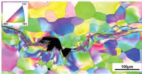
Pores and pore coalescence in dynamically loaded Tantalum
