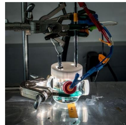
Solar simulator and photoelectrochemical cell for testing light harvesting by thin-film electrodes
