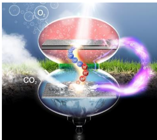
Schematic illustration of an integrated solar-driven CO 2 reduction prototype
