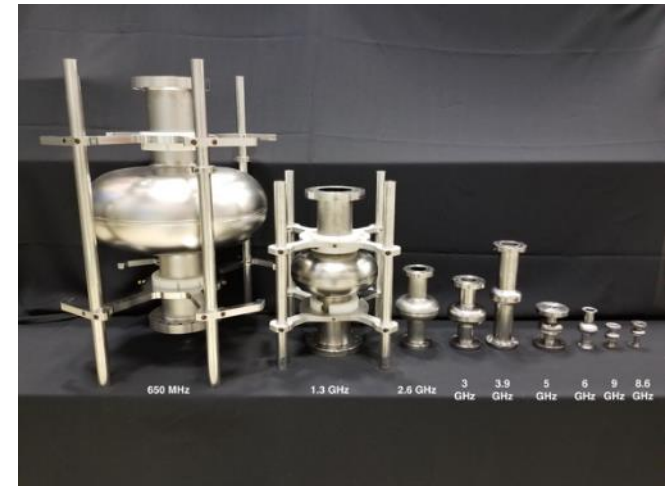
Development of smaller cavities for higher frequencies pave the way towards dramatic improvement of qubit coherence time
