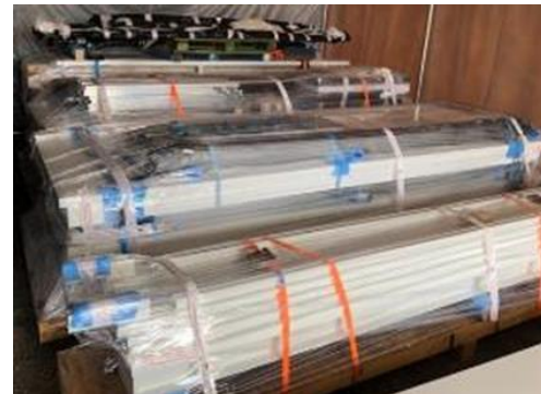
Shielded enclosure panels
