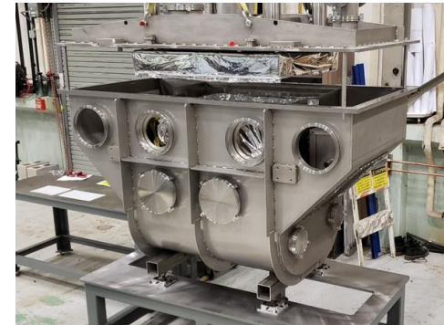
SC bunch lengthening cavity cryo-vessel
