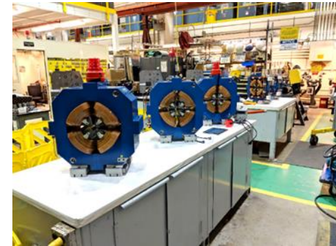
Production Q1 quadrupoles
