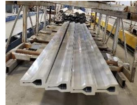
ID chamber extrusions
