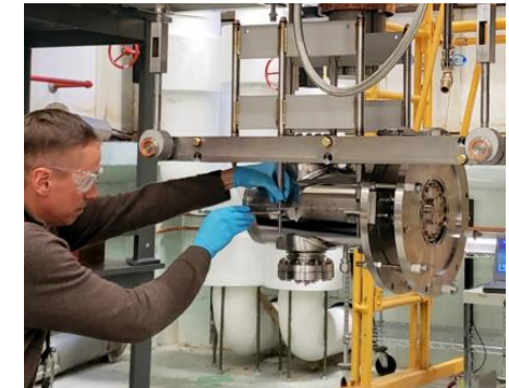
SC bunch lengthening cavity
