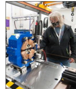
Kris Meitsner tests a quadrupole magnet during COVID using ANL safety protocols.
