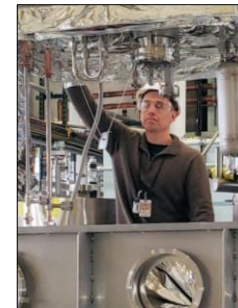
Mike Kelly checks & prepares APS-U Super Conducting Cryovessel at ANL.
