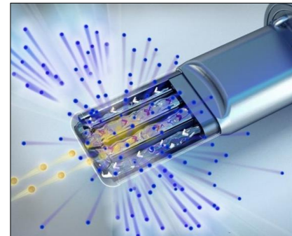
Protons (yellow) strike the liquid Hg target creating neutrons by spallation.
