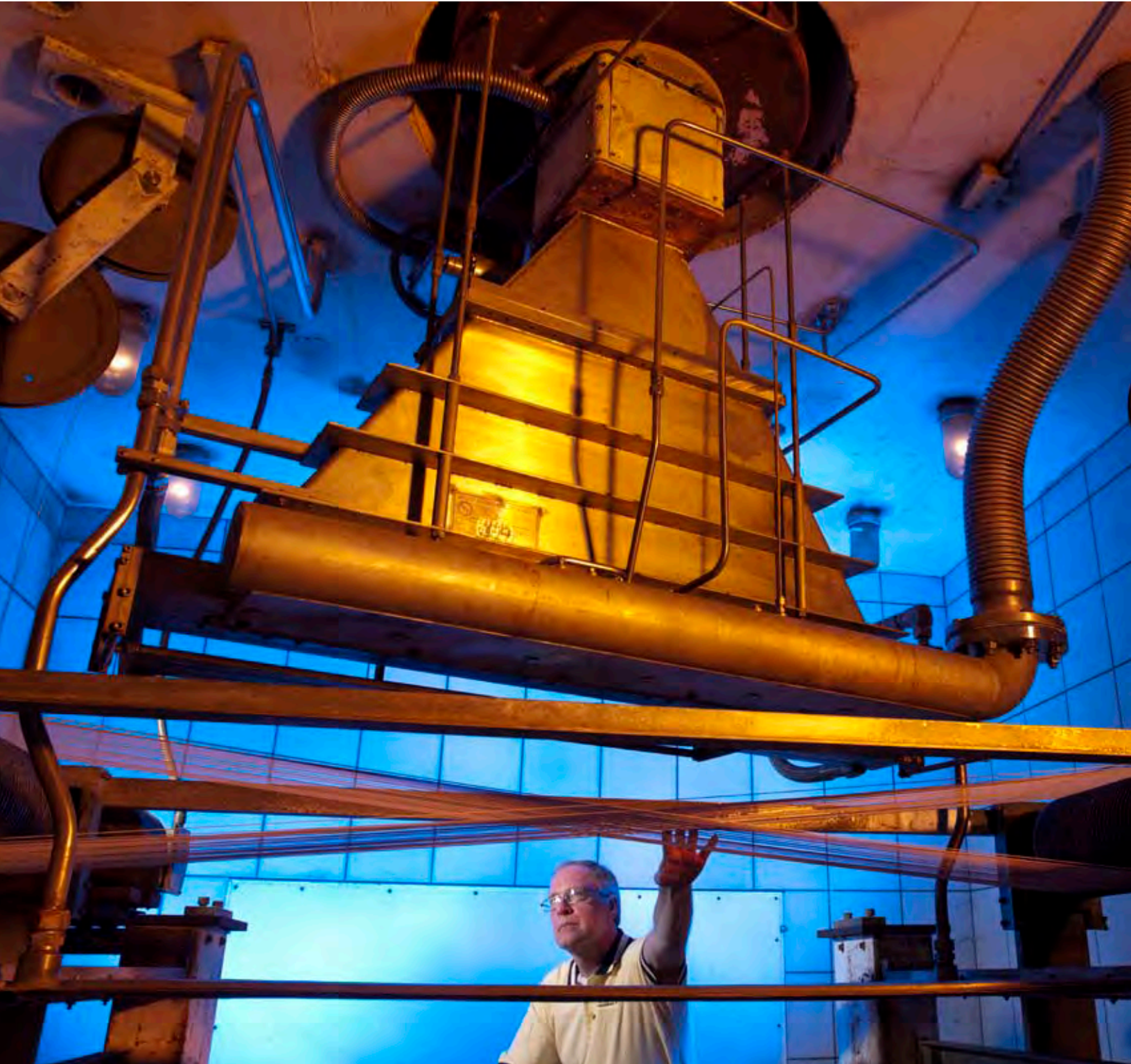
Crosslinking of polymers by an electron beam, as in this Illinois plant, improves heat resistance of coatings for wire and cable. Photo: Reidar Hahn, Fermilab
