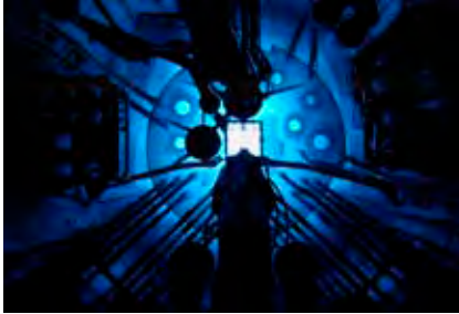
The high-energy beta particles from spent nuclear fuel give rise to a blue glow known as Cerenkov radiation. Photo courtesy of Australian Nuclear Science and Technology Organisation
