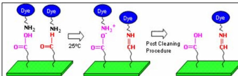
Figure 1 Chemical Specificity of FLOSS. The post reaction cleaning is effective in removing ionic dyes from the surface. The presence of carboxyl groups on the surface does not affect detection of aldehyde groups using amino modified dyes.
