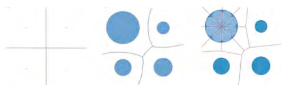
Figure 1. Schematic depiction of Voronoi tessellation around four particles: (left) “standard” Voronoi around point particle, (center) tessellation with curved boundaries around atoms of unequal radii, (right) tessellation after replacing the largest atoms with a cluster of smaller atoms.
