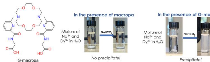
Figure 3. Structure of G-macropa and photographs showing how its presence can lead to selective precipitation of Dy 3+ from an aqueous solution containing both Nd 3+ and Dy 3+ .
