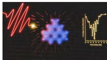
Figure 1: Schematic of a IR pump/X-ray probe of transient metallization in diamond. Our simulations use time-dependent density functional theory simulations with bulk-mimicking clusters.
