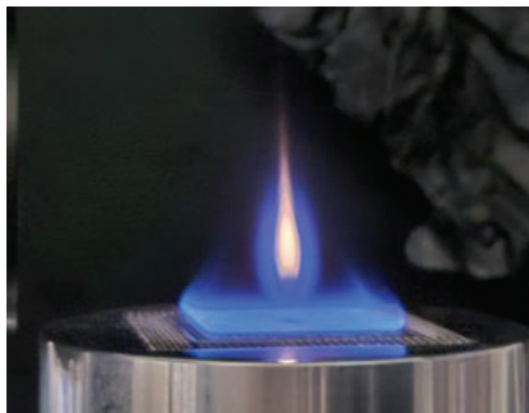
Figure 7. Image of nanoparticles being produced in the diffusion flame created when HMDSO precursor is introduced via an inert gas jet in the center of the MEDB. The primary flame is a lean ( \phi = 0.8 ) methane and air flame.
