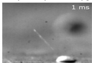
Figure 4. High speed photography image of aerosol formation during cellulose pyrolysis.
