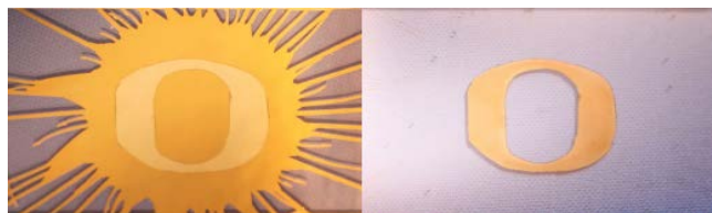
Figure 3. Sulfonate functionalized polyacetylene ionomer with tetramethylammonium (O-shaped region) and \text{Na}^+ counter ion immediately after ion exchange (left) and after 15 days under photo-oxidative conditions (right).
