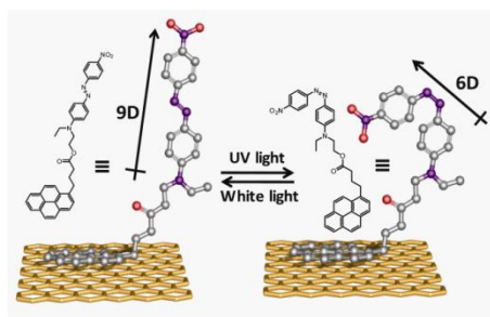
Figure 3. Illustration of photoisomerization of DR1P on graphene. DR1P is tethered to the surface of graphene via \pi - \pi interactions between
