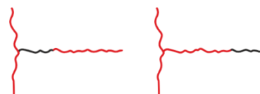
Figure 8. Specifically labeled bottlebrush polymers with inner part (left) and outer part (right) highlighted.
