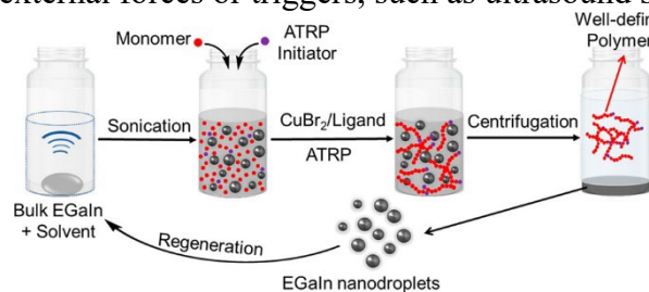
Figure 3. A typical procedure of ATRP in the presence of EGaIn micro/nanodroplets.
