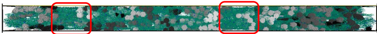
Figure 12. Snapshot of a simulation illustrating formation of voids in particle-poor regions that evolved during earlier deformation stages. Red outlines highlight two major cavitation regions, with the cavities in these regions spanning the period boundaries of the box.
