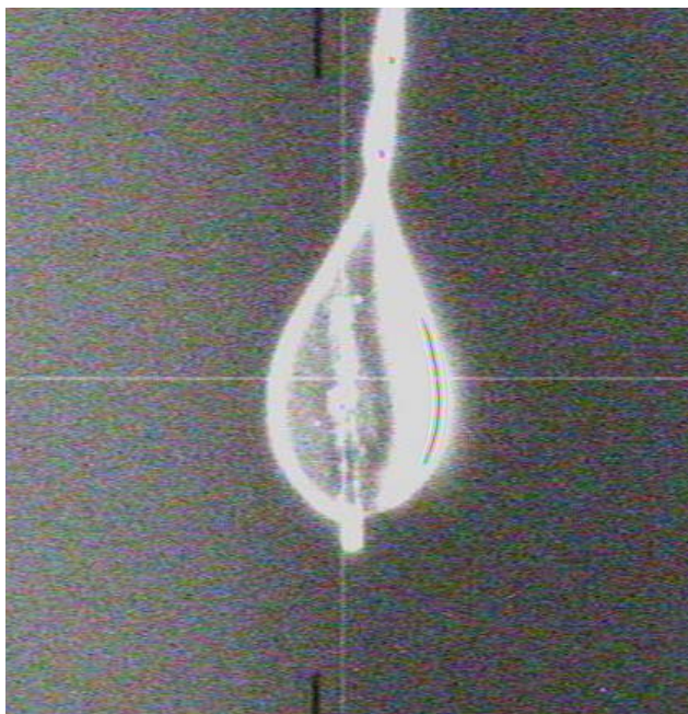
Fig. 1. Nylon loop filled with a thin layer of cryo-protecting oil with the ribbon attached to it. The ribbon is clearly seen as the vertical bend; X-ray beam hits at the intersection of the two hair-lines. The ribbon width is of 50 microns, similar to the cross-section of the X-ray beam.
