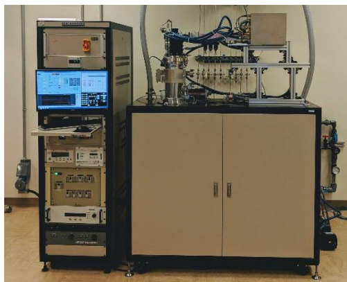
Figure 1 | Seki SDS6300 diamond microwave-assisted plasma-enhanced chemical vapor deposition (PE-CVD) tool at ANL.
