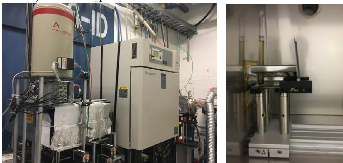
Figure 4. Left: A custom-built class-A convection oven for reproducible solvothermal reactions, with beam ports on each side, in place at Advanced Photon Source beamline 6-ID for energy-dispersive X-ray diffraction (EDXRD) of \text{Cu}_4\text{O}_3 formation in ethanol-DMF. Right: The reaction tube inside the oven, with beam port on left marked by a square of Kapton and mylar tape.
