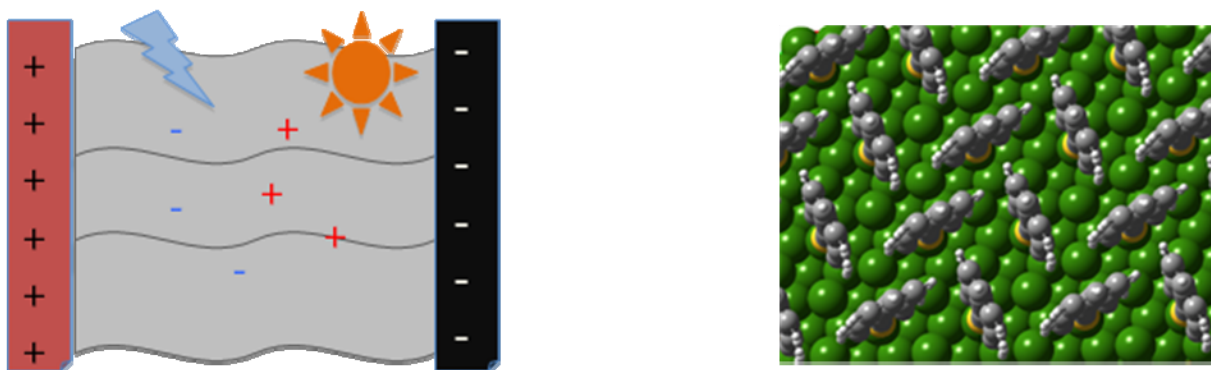
Figure 5. New photovoltaic materials require understanding organic-inorganic interfaces brought about by more sophisticated methods for modeling light-matter interactions and for calculating transfer of energy from a collective many-electron excitation to an activated adsorbate. Image courtesy of Hai-Ping Cheng (University of Florida/Quantum Theory Project).
