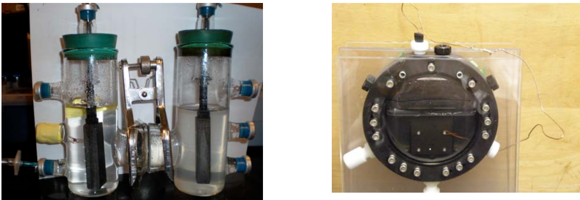
Figure 1: Microbial fuel cells established with Fe-reducing bacteria: left, standard cells and right, newly designed cell optimized for the current research.
