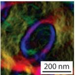
Specialized transmission electron microscopy of magnetism, in combination with simulations, allows observation of skyrmion formation, behavior, and stability..
