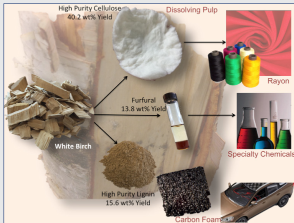
Sidebar Figure 1.1. Reprinted with permission of Alonso et al., "Increasing the Revenue from Lignocellulosic Biomass: Maximizing Feedstock Utilization," Science Advances , 2017. Copyright © 2017 Alonso et al.
