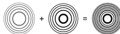
Schematic depiction of double-patterning process. (W. Chao et al., J. Vac. Sci. Technol. B 27 , 2606, 2009)
