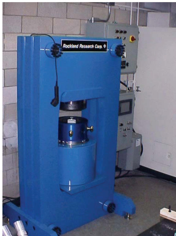
Figure 2 High Pressure Anvil Furnace; max. p = 60 kbar; max. T = 1000 °C. [R. Cava, Princeton U.]
