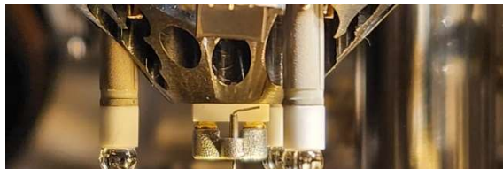
Figure 13: Scanning Tunneling Microscope probe at ASU to be used as a new method to investigate DC field emission from alkali-antimonides.
