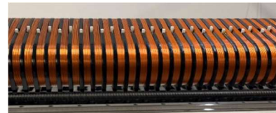
A 1 m long prototype of the undulator magnet has been measured in a vertical cryostat.
