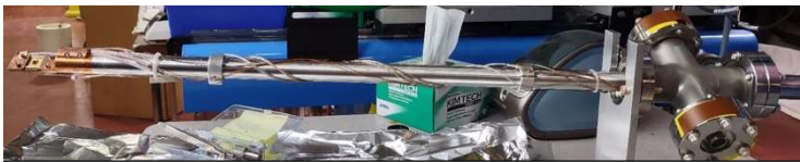
Fig. 3. A probe capable of measuring various transport properties with provisions for cryogenic cooling.
