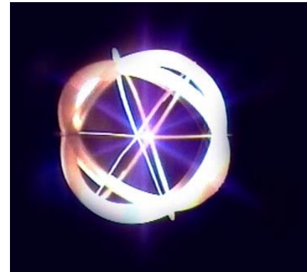
Fig. 3.4. Commercial IEC neutron generator.
