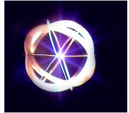
Commercial IEC neutron generator from < http://www.dasa.com/fusionstar >
