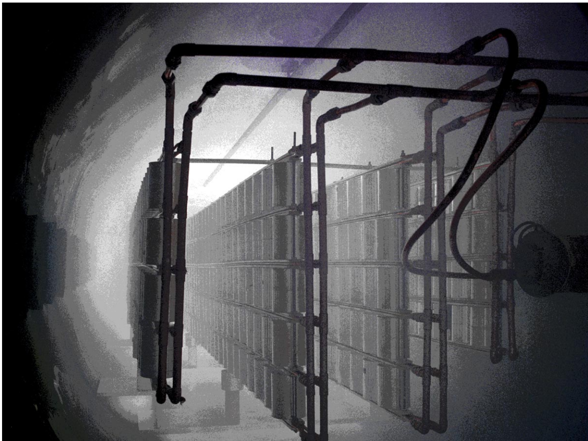
Fig. 4.4. Plasma cleaning, ion implantation, and DLC deposition of 1000 automotive pistons in a former OFES facility.
