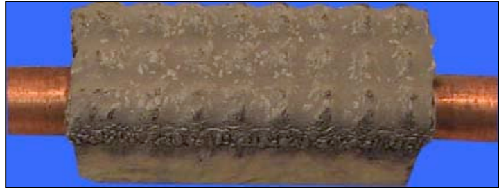
Figure 6.4. Mock-up of an ITER first-wall component fabricated by plasma spray of beryllium onto a copper alloy heat sink ready for high-heat-flux testing. (Courtesy of D.Youchison, SNL, and K.Hollis, LANL)
