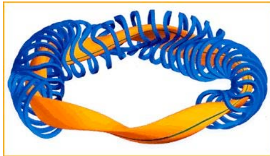
Fig. 4-3. W7-AS modular non-planar coils and plasma.
