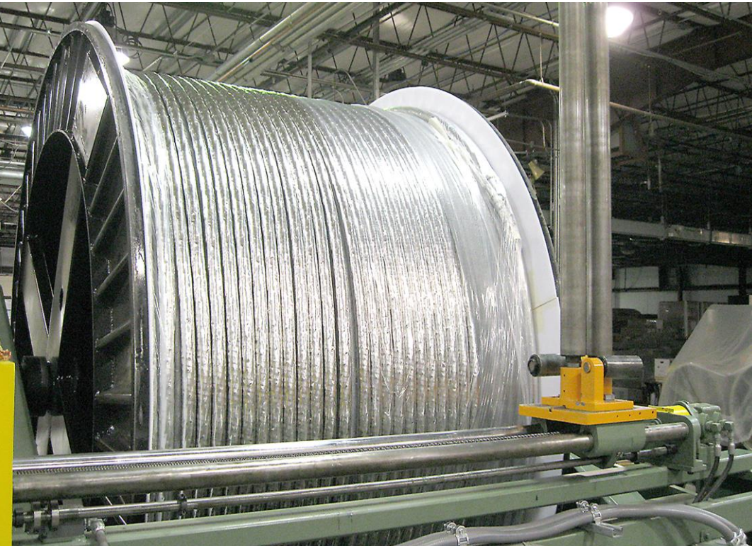
Production conductor cabled at New England Wire Technologies in Lisbon, NH
