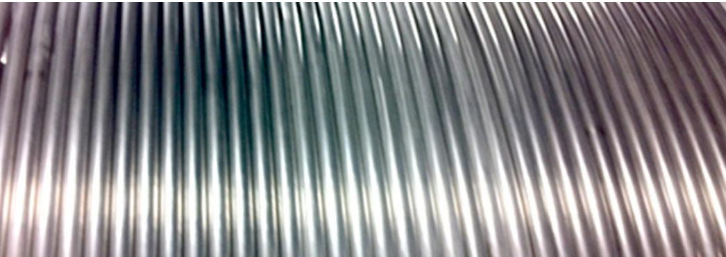
Close-up view of the Oxford 100 m active conductor before packaging . Photo: US ITER
