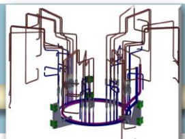
9: Helium Piping & Measurement
