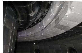
Reshaped upper divertor tiles – SAS divertor to increase closure
