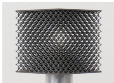
Figure 4.3.1. Rhombic dodecahedral lattice structure made of 316SS using SLM. Photo courtesy of LLNL.
