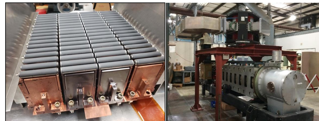
Helicon antenna modules and 1 MW klystron from SLAC
