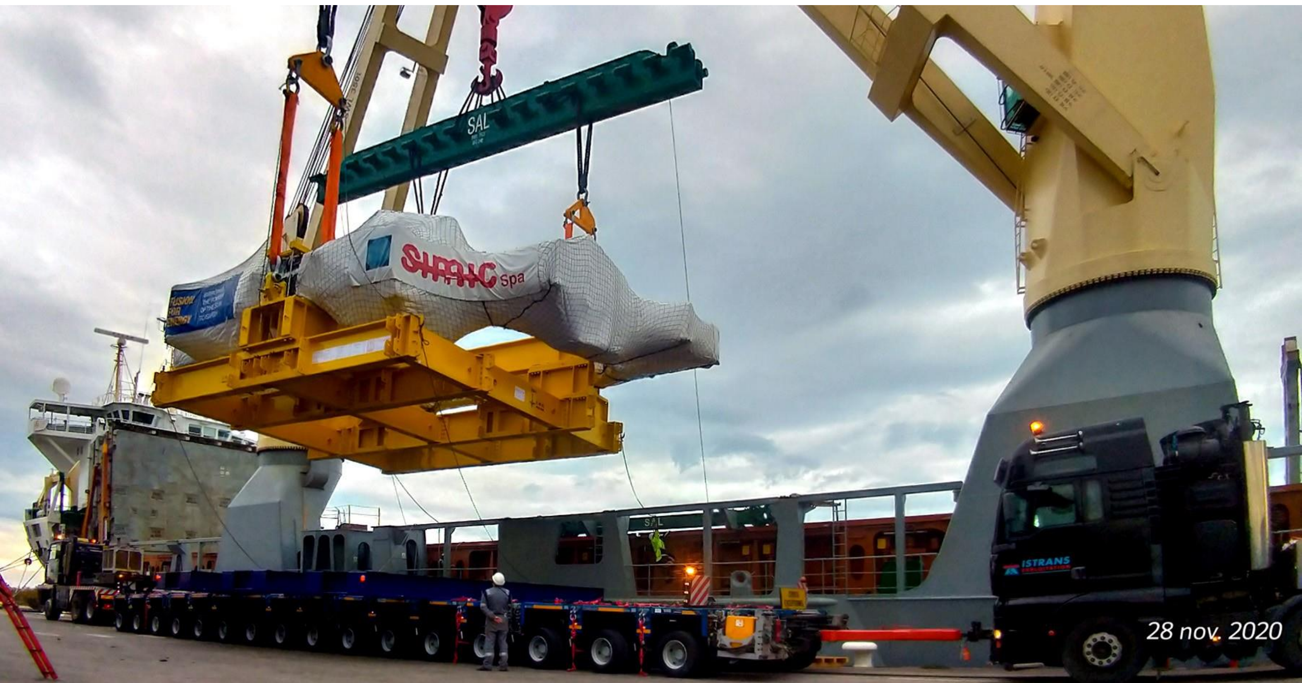
Delivery of D-shaped toroidal field coil #5 (of 18) at Fos Harbor, being loaded onto modular transporter for journey to ITER site
