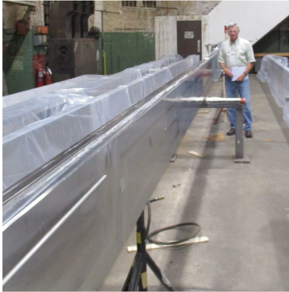
Inner tie plate during cryogenic shock testing at PCC.
