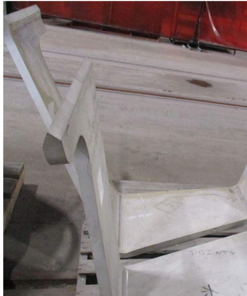
Upper feeder brackets during forming at PCC.
