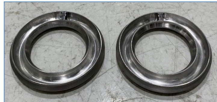
Weld plugs antenna cap
